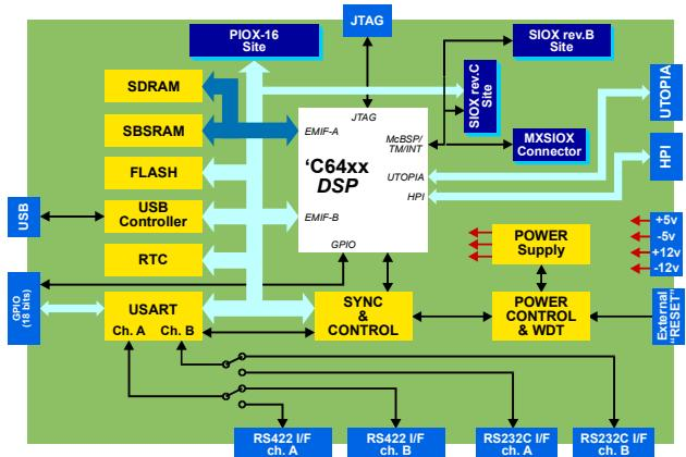
**TORNADO-E64x** are ultra-high performance embedded DSP controllers with the industry standard 3U form-factor for real-time data acquisition and DSP. Flexible modular construction and a variety of “off-the-shelf” AD/DA/DIO and I/O coprocessor expansion daughter card modules make **TORNADO-E64x** an ideal selection for embedded telecommunication, telephony, multimedia, acoustics, instrumentation, digital radio and many more application.
