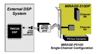
side and to MPSD/JTAG emulation interface of target TMS320 DSP on the other side.
