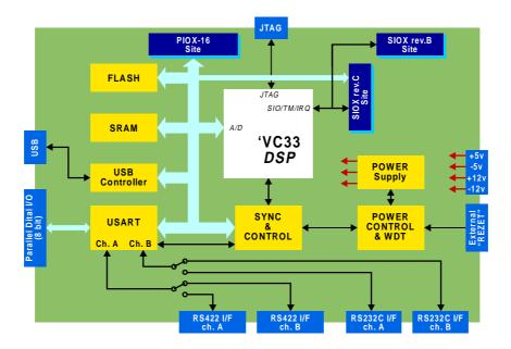
TORNADO-E33 is a high performance floating-point embedded DSP controller with the industry standard 3U form-factor for real-time data acquisition and DSP. Flexible modular construction and a variety of "off-the-shelf" AD/DA/DIO and I/O coprocessor expansion daughter card modules make TORNADO-E33 an ideal selection for embedded telecommunication, telephony, multimedia, acoustics, instrumentation, digital radio and many more application.
